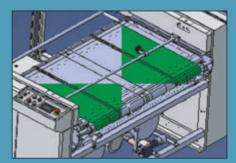
The broad conveyor belts assure stable delivery of prints to the stack board.
