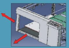
Pallet with piled sheet can be pulled out to the rear way as well as either side way subject to the space available.
